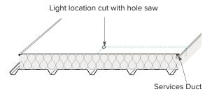
Feed electrical conduit through Services Duct to fan or light location.
