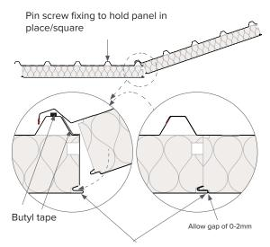
Pull it down and engage the male interlock into the female interlock of the ceiling side of the first pane.
