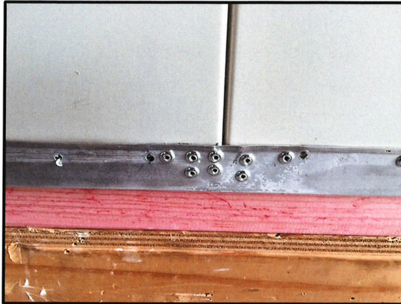
Image 2: Strengthening of joint region of 2.4m long Metalcraft test panel.
