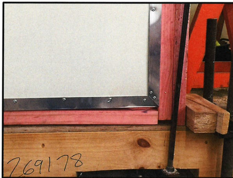
Image 1: End region uplift and yielding of bottom aluminium angle:
